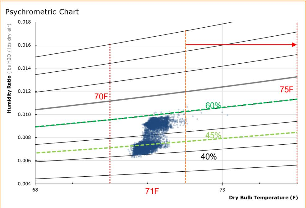
With expanded operating parameters moisture tends to be more spread, up to 60% down to 40% RH.
