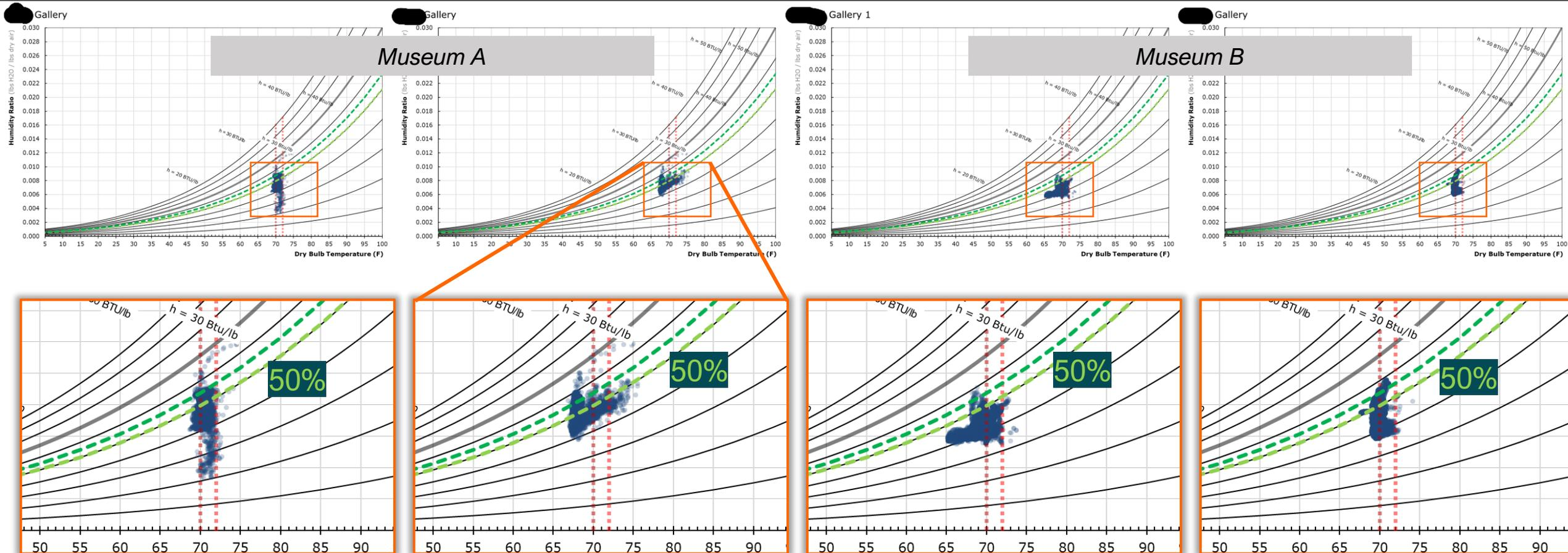
Logger data from two field sites for different galleries shows a spread of operating conditions around 70°F and 50% RH, most sites maintaining 68–72°F. Moisture values show at or below 50% RH with several sites at 40% RH frequently.
