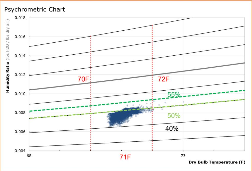
Similar results from the model as observed in field sites, temperature is maintained, moisture tends to be at or below the setpoint.
